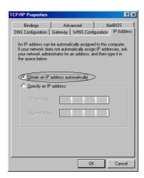
For Fixed IP or DHCP server, Click the IP address tab, and click the Specify an IP address button. Then set IP Address and Subnet Mask to the same subnet as remote host. Refer to Chapter 3.2 for example.
